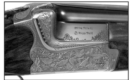
Wood-to-metal fit on our sample was excellent—a testament to the inletting skill of the stockmaker considering the difficulty of mating the action to the buttstock.
