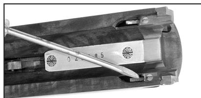
Small slotted screws are incorporated into the fore-end iron to disable the ejector sears. Rotating the screws 90 degrees converts the automatic ejectors to extractors.
