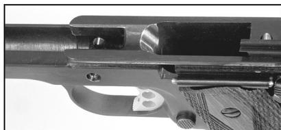
All Rock River frames are machined to tight match tolerances from 4140 steel forgings. The feed ramp (above) is polished and our sample pistol fed and functioned flawlessly with semi-wadcutter ammunition.
