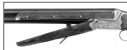
The Merkel 2001EL's fore-end is the traditional Suhl three-piece style, the bottom of which is secured by a Deeley-type latch and covers only part of the gun's bottom barrel.
