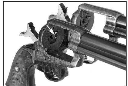
The cylinder hand (arrow) on the Colt Cowboy (l.) is different from that of the SAA. Note also that the new Cowboy lacks the firing pin bushing on the recoil plate.
