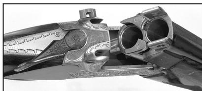
Lockup remains the Kersten crossbolt system, which is a modification of the Greener crossbolt lock. Square lugs with centrally located round holes extend back from the top of the over barrel into corresponding cuts in the gun's standing breech.
