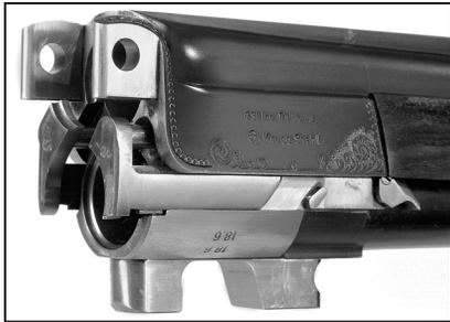
**Barrel joining is by the demi-block system in which each has a solid, forged breech section. The over barrel's breech is shaped like an inverted U, with the lower barrel fitting into a squared recess in its bottom.**
